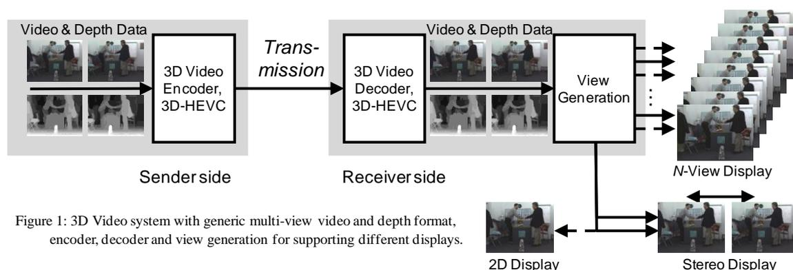
Figure 1: 3D Video system with generic multi-view video and depth format, encoder, decoder and view generation for supporting different displays.
