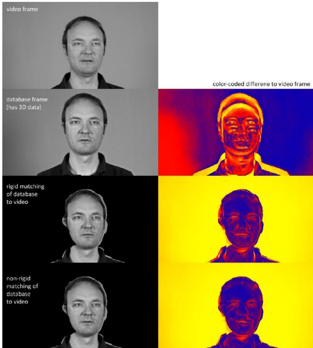
Figure 8 Matching of a database image, capture at the pre-modelling stage, to a video frame from a PTZ camera
