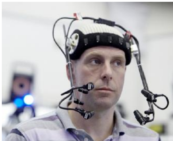
Illustration 2, example of head-mounted system used to capture actors' expressions. Visible in front of the actor's face are four cameras arranged as two stereo pairs.
