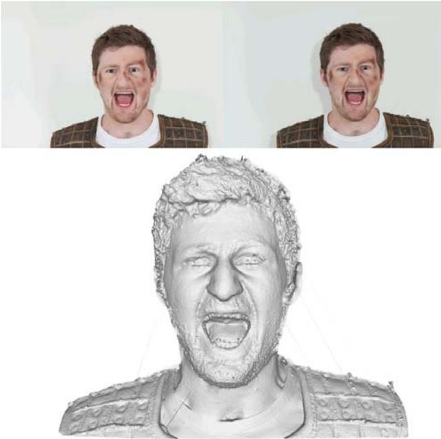
**Figure 1: Example reconstruction result: stereo input image pair and result of our 3D reconstruction method.**
